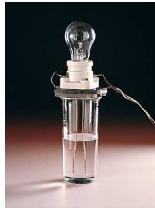
Sugar and Water; No Ions present; electricity is not conducted – bulb off.
