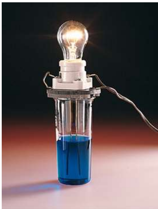
CuSO_4 and Water; Ions present; electricity is conducted – bulb on.
